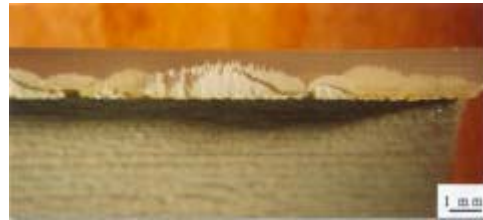
Figure 4: Axial Cross-section of PEX Pipe Material.
