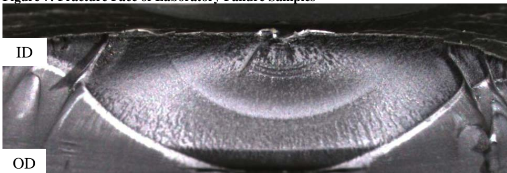
Figure 7: Fracture Face of Laboratory Failure Samples
