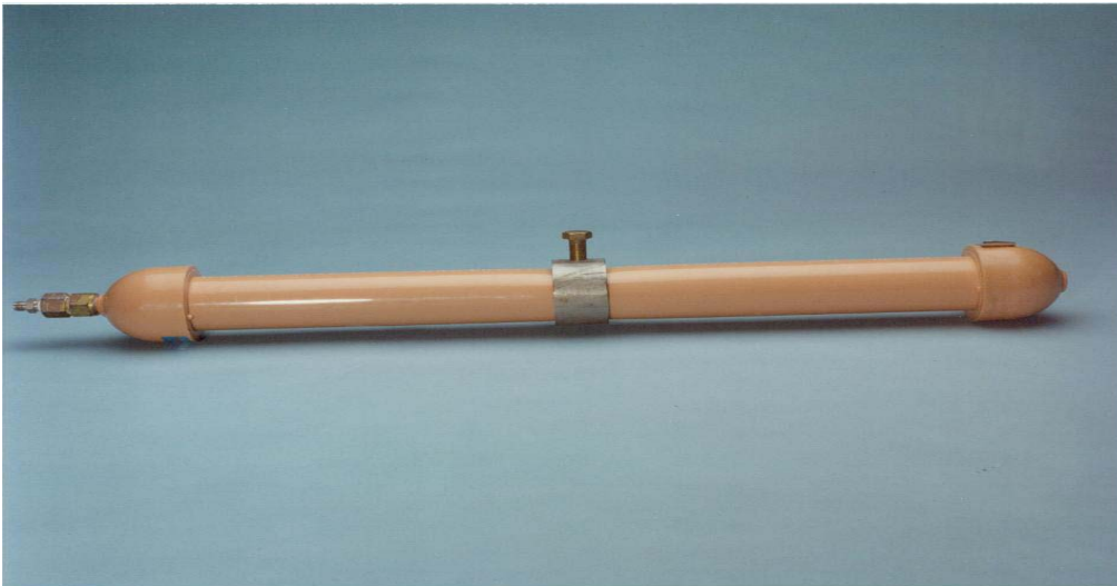
Figure 2: Indentation Jig for Simulation of Rock Impingement
