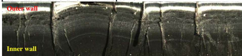
Figure 1: Typical Fracture Face of an Un-Notched Specimen
